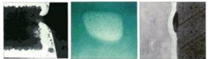
Corrosion due to ionic contaminants, popcorning
