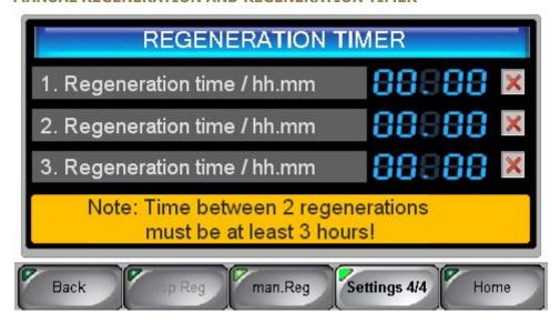
Continue to the fourth setting page by pressing [Next]. This page contains the regenerations timer. Here you can define up to three times, in which a regeneration is to be started. Dynamic regeneration remains active so that additional generations are performed automatically. If this is not desired, the dynamic regeneration on the service menu has to be deactivated.
