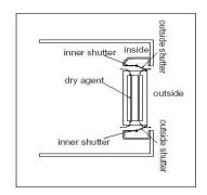
Every drying cabinet has contact switches installed on each of the doors to control a fan inside the electric drying unit. The interlocked fan operates for about 2 hours after the drying agent is rejuvenated in order to accelerate moisture absorption. The interlock fan stops when the door is opened to minimize inflow of ambient air into the unit. The interlock fan will operate for 20 minutes when the doors are closed to speed up moisture absorption inside the drying cabinet.
